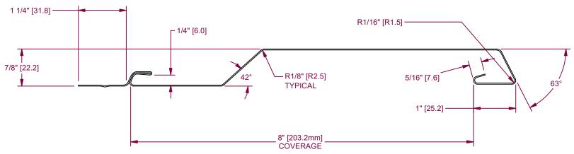
ALTERNATE HEM FOR CLIP DECREASE COIL WIDTH BY 1-3/4" [44.5mm]
