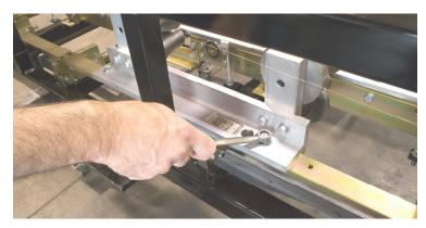
Figure 50: Removing Tooling Rails
