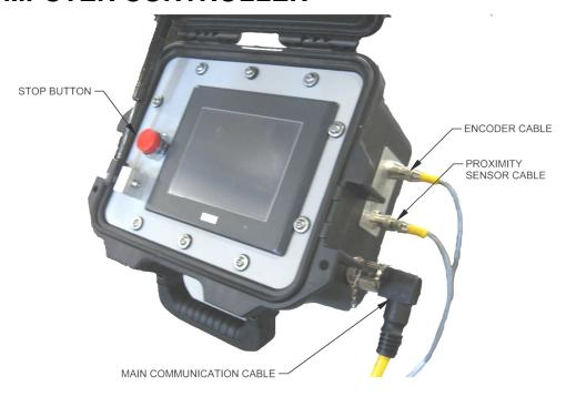
Figure 109: Computer Controller Assembly
