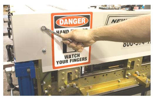
Figure 64: Removing Shear Cover
