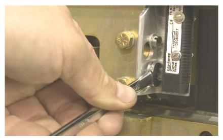
Figure 60: Removing Photo Eye and Bracket (If Equipped)
