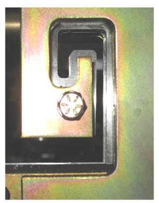
Figure 39: Exit Die Adjustment
