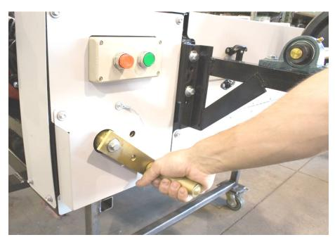
Figure 24: Tooling Rail Adjustment Handle
