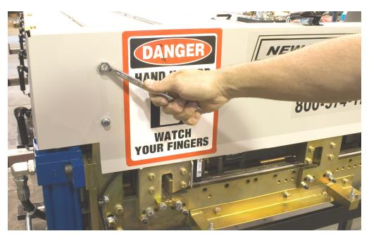
Figure 59: Removing Shear Cover
