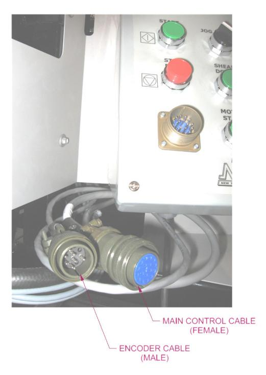
Figure 6: Control Cables
