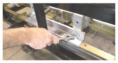
Figure 41: Removing Tooling Rails
