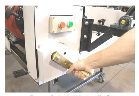
Figure 54: Tooling Rail Adjustment Handle
