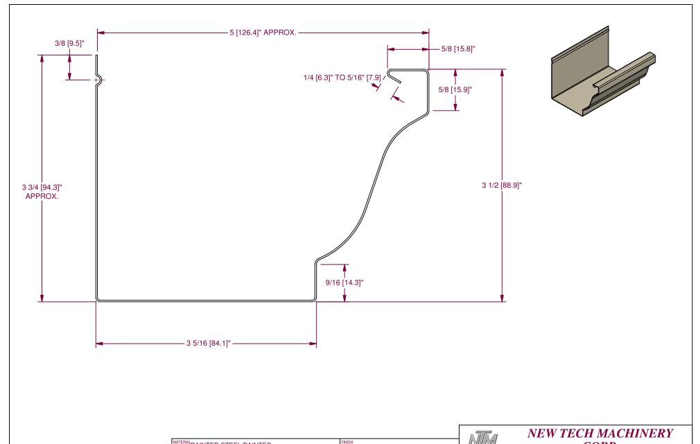
NOTE: 1. COIL WIDTH: 11 3/4" [298mm] to 11 7/8" [302mm] 2. DUAL DIMENSIONS: Inch [mm]
