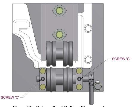
Figure 81: Bottom Bead Roller - Disengaged
