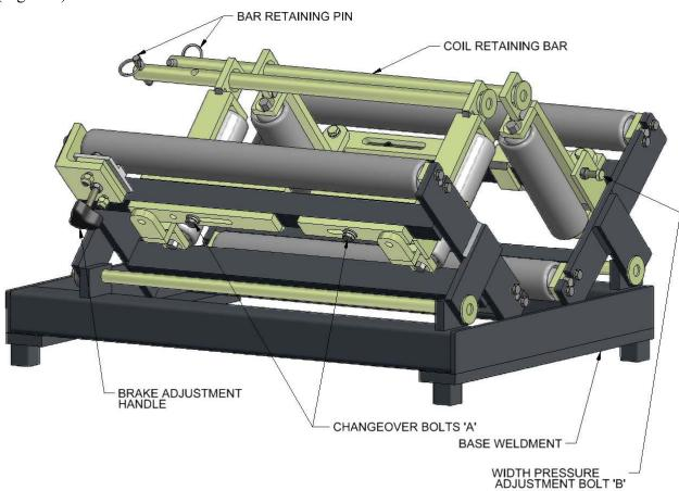
Figure 8: Cradle Assembly (5" Position Shown)
