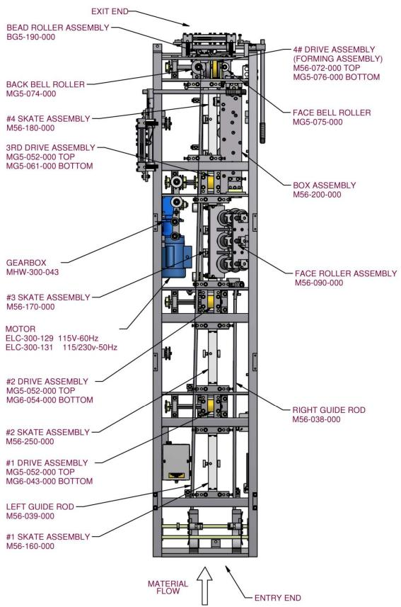
Figure 4: M56 Machine Layout
