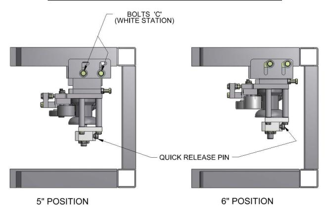
Figure 52: Combo Box Assembly Positions
