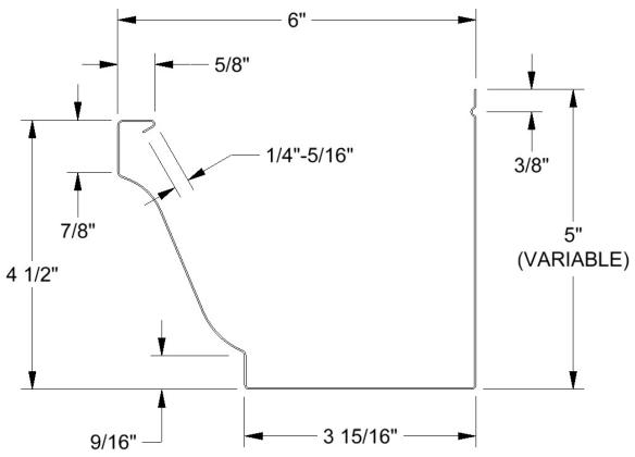
Figure 85: 6" Gutter Profile
