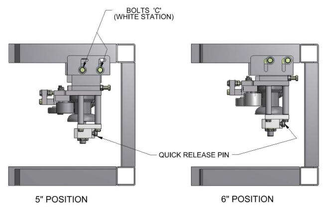
Figure 69: Combo Box Assembly Positions
