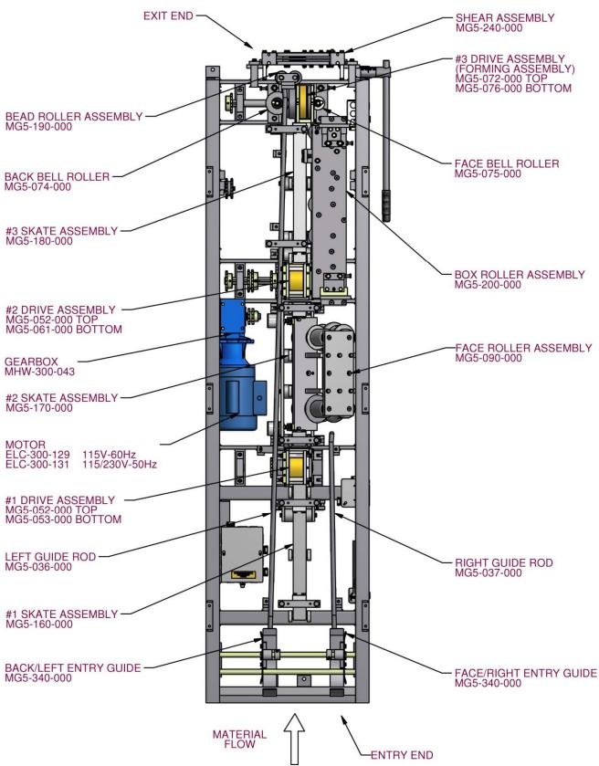
Figure 2: MG5 Machine Layout
