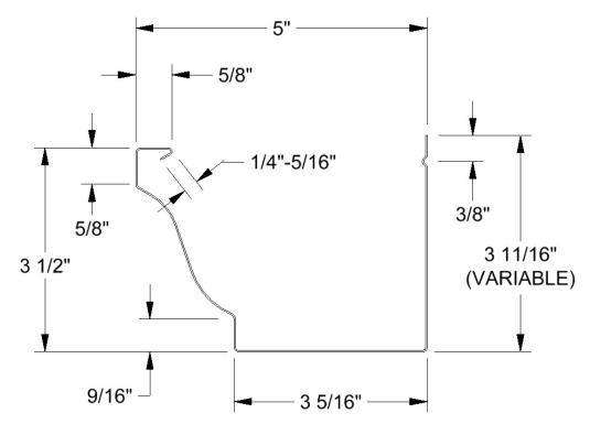
Figure 84: 5" Gutter Profile
