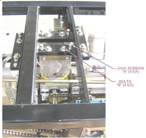
Figure 21: Top Drive Pressure Adjustment Screws
