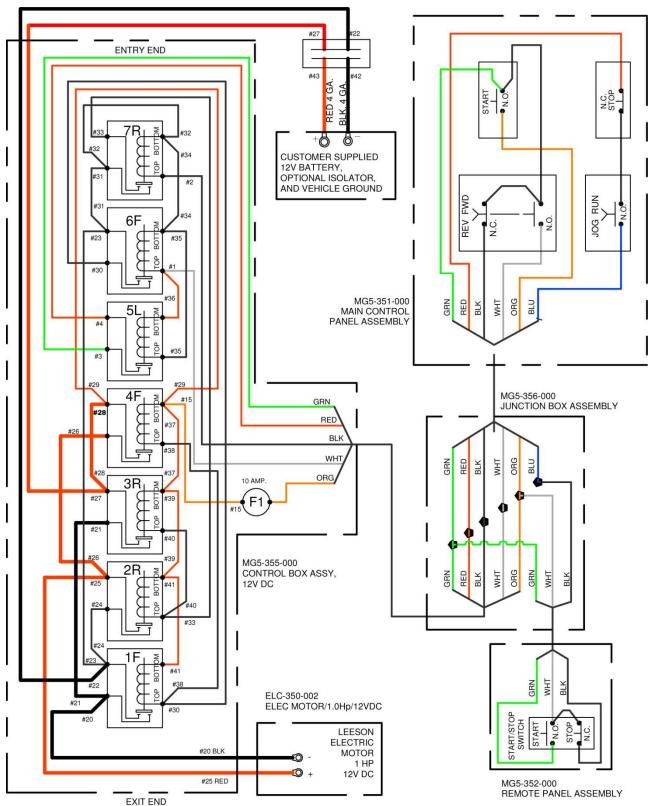
Figure 92: MG12V – 12VDC Wiring Diagram
