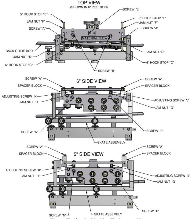
Figure 77: Combo Machine Hook Assembly
