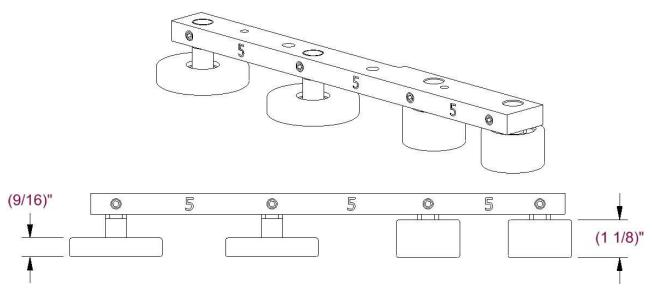
Figure 53: 5" Roller Bar
