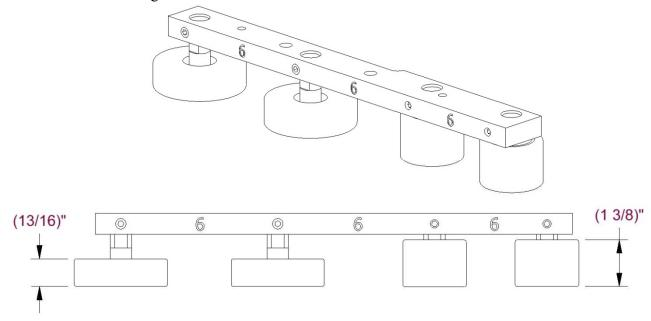
Figure 54: 6" Roller Bar
