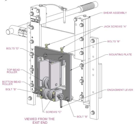
Figure 82: Bottom Bead Roller Assembly
