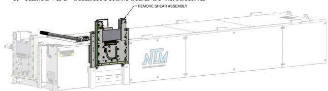
Figure 57: Remove 5" Shear
