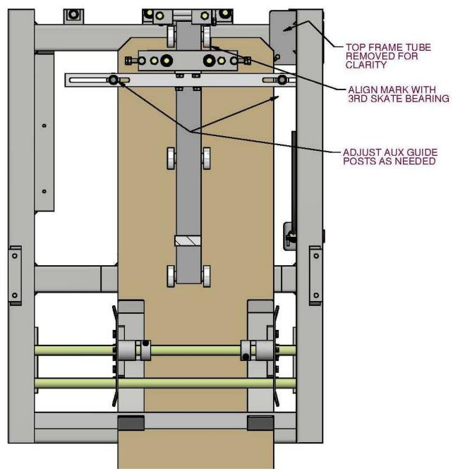
Figure 20: Feeding Material - 3rd Skate Bearing
