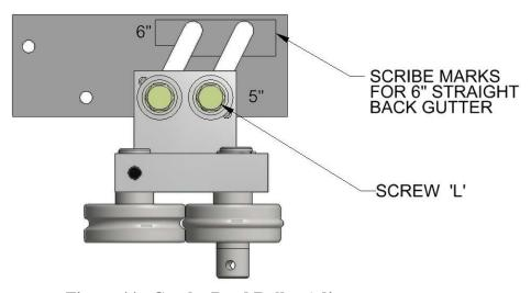
Figure 44: Combo Bead Roller Adjustment
