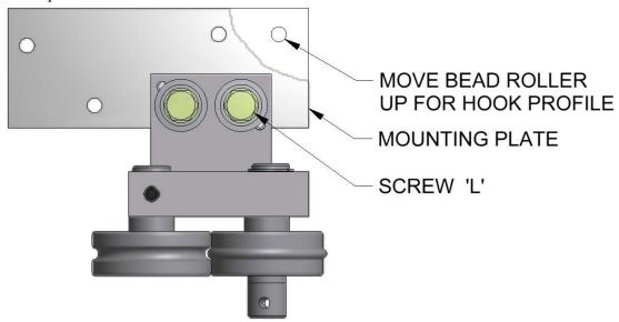
Figure 74: Bead Roller Assembly - MG5
