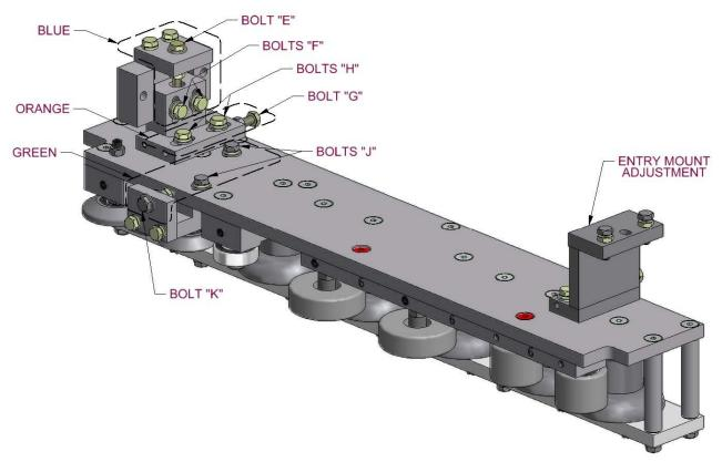
Figure 23: Gutter Box Assembly
