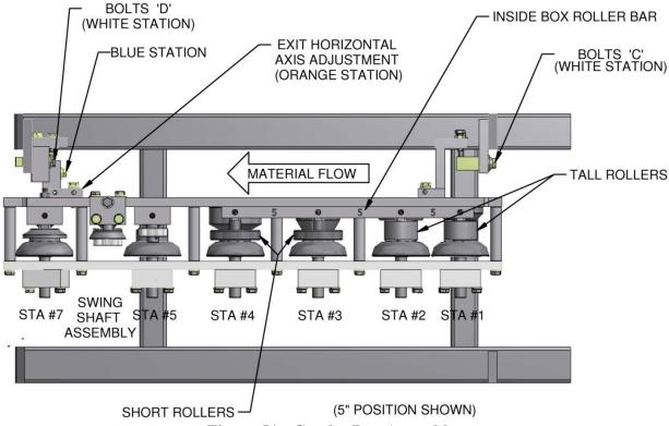
Figure 51: Combo Box Assembly
