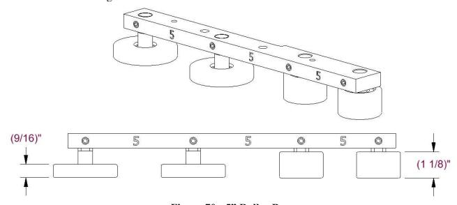
Figure 70: 5" Roller Bar
