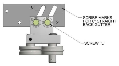
Figure 62: Combo Bead Roller Adjustment
