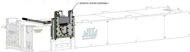
Figure 41: Remove 6" Shear
