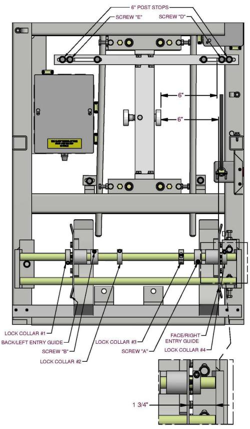
Figure 18: M56 Entry Guide Setup for 6"
