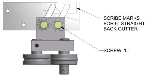
Figure 78: Bead Roller Assembly – M56 (Shown in 5" Position)
