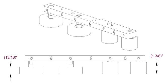
Figure 67: 6" Roller Bar
