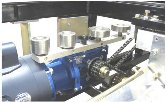
Figure 55: Unused Inside Box Roller Stored
