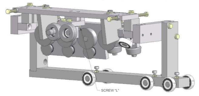
Figure 79: Bead Assembly Stored
