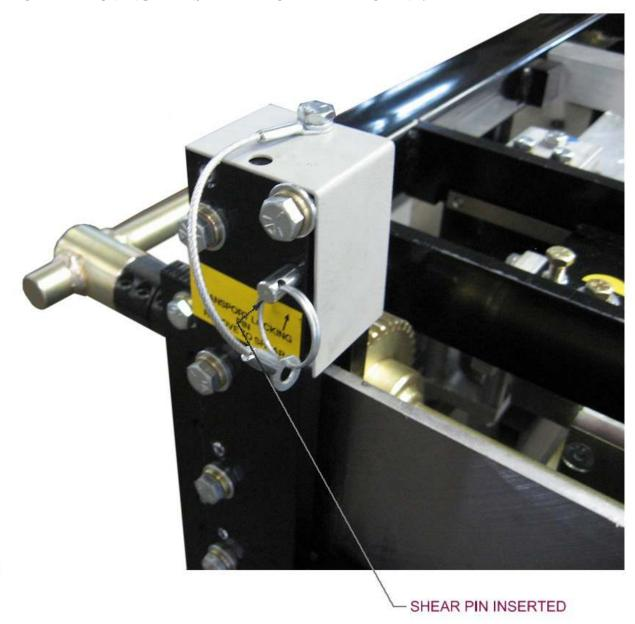
Figure 59: Shear Pin
