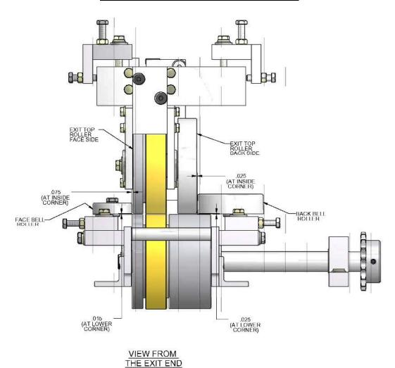
**Figure 29: Exit Drive Clearances**
