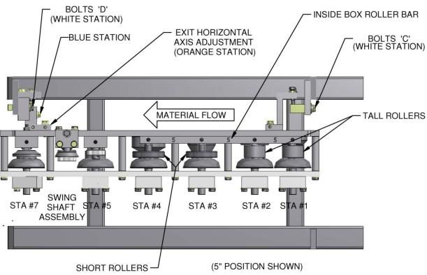
Figure 68: Combo Box Assembly
