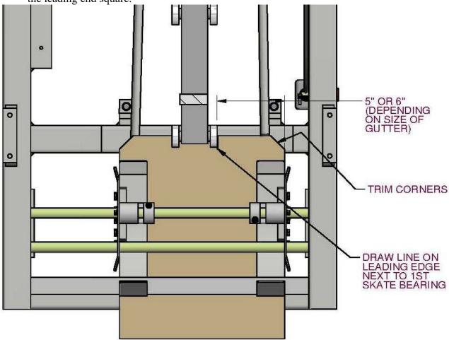
Figure 19: Feeding Material – 1st Skate Bearing
