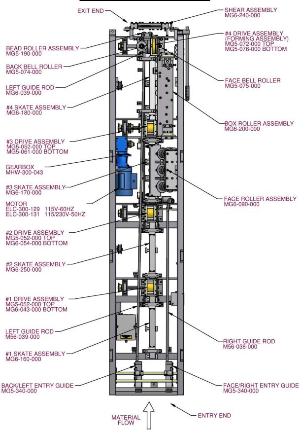
Figure 3: MG6 Machine Layout
