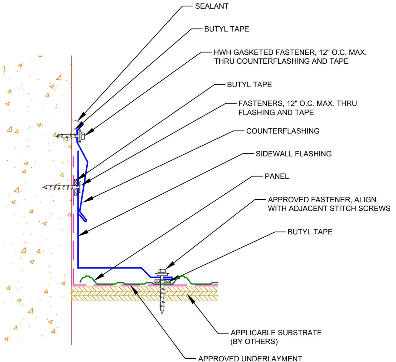
**NOTE:** 6" MIN. LAP ON SIDEWALL FLASHING WITH APPROVED SEALANT IN LAPS.
