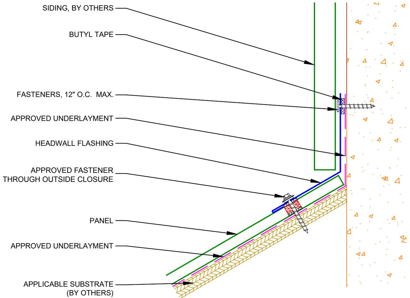
NOTE: 6" MIN. LAP ON HEADWALL FLASHING WITH APPROVED SEALANT IN LAPS.
