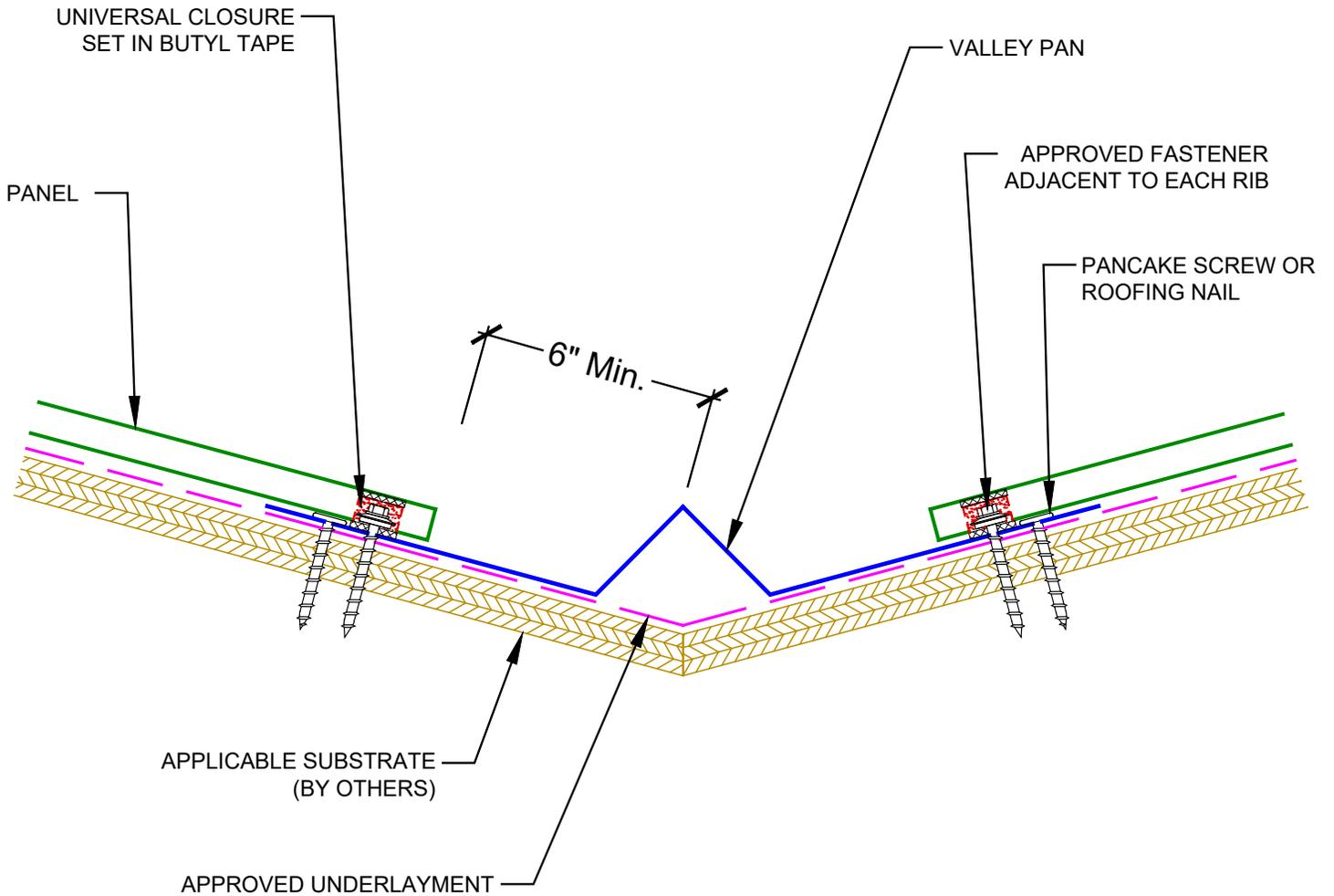
NOTE: FLASHING LAPS IN VALLEY ARE 6" MIN. USE TWO ROWS OF APPROVED TUBE SEALANT IN ALL LAPS.
