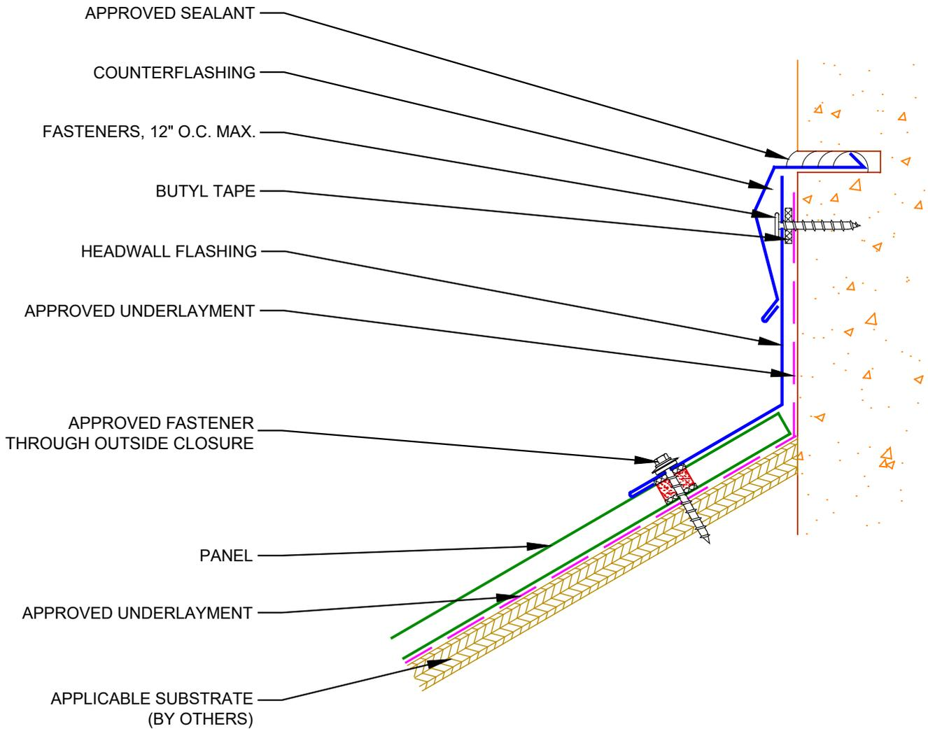
NOTE: 6" MIN. LAP ON HEADWALL FLASHING WITH APPROVED SEALANT IN LAPS.
