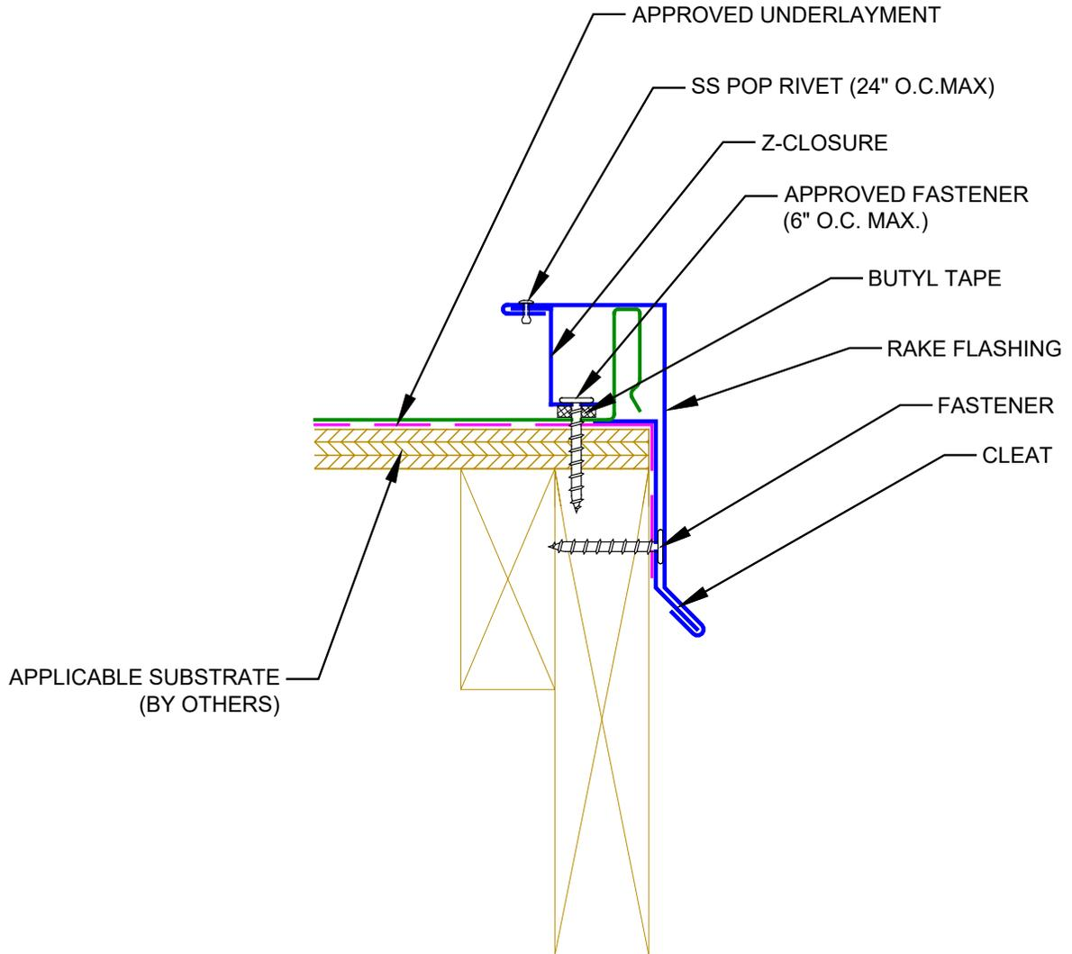
**NOTE:** 4" MIN. LAP ON DRIP EDGE WITH APPROVED SEALANT IN LAPS.
