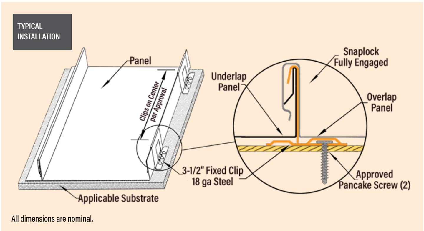
**!** Actual clip and fastener pattern may vary from the pattern shown based on the specific roof plan, metal type and strength, local building codes and product approvals.
