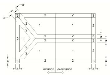
a: 10% OF LEAST HOIZONTAL DIMENSION OR 0.4h, WHICHEVER IS SMALLER, BUT NOT LESS THAN EITHER 4% OF LEAST HORIZONTAL DIMENSION OR 3FT (0.9M), OR AS DETERMINED BY DESIGN OR OTHER APPLICABLE CODE.
